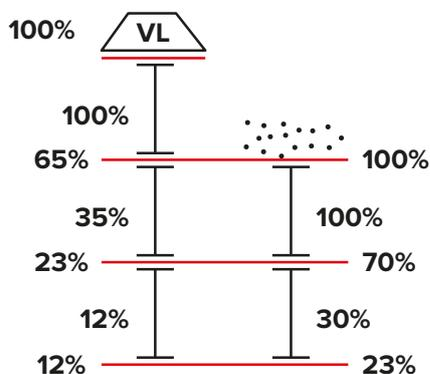
Two levels of back props keeps the load spread prior to the reinstatement of the props at the level below.
